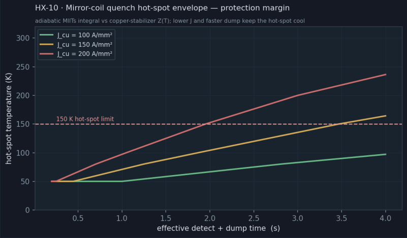
Hot-spot temperature vs detect+dump time for three stabilizer current densities.
