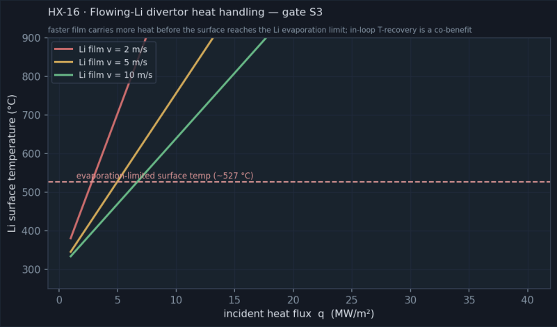
Li surface temperature vs incident heat flux for three film velocities.
